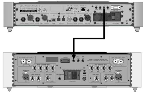
Figure 4: Remote Operation with SimLink™
