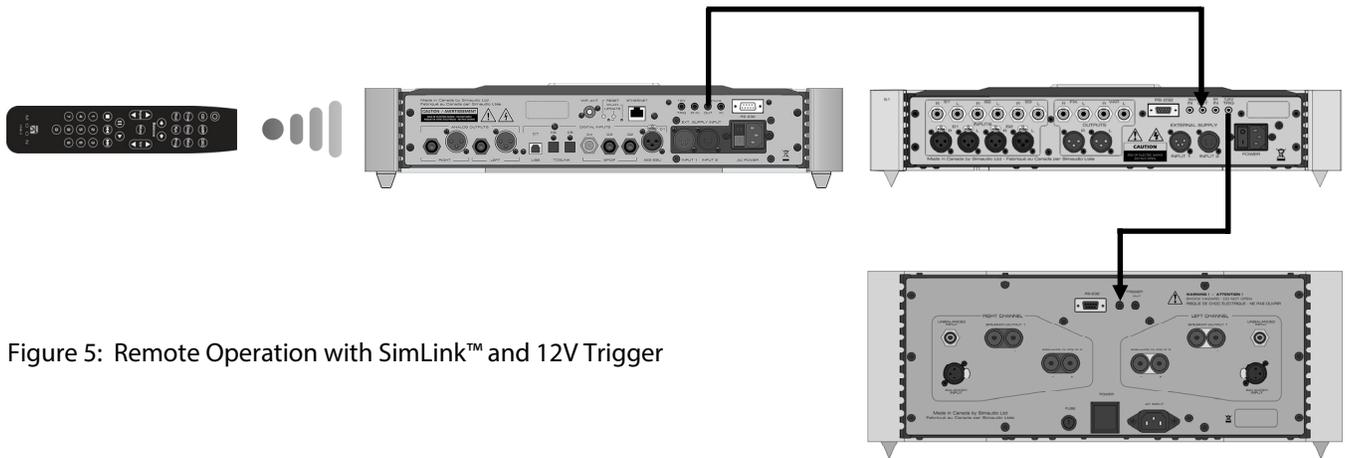
Figure 5: Remote Operation with SimLink™ and 12V Trigger
