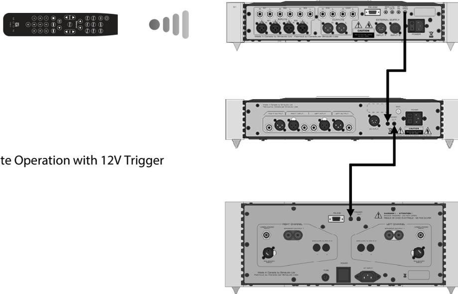
Figure 8: Remote Operation with 12V Trigger
