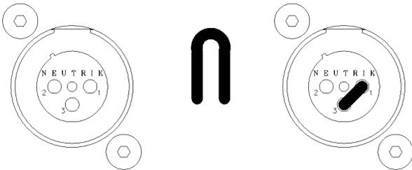
Figure 7: XLR connector without and with jumper accessory
