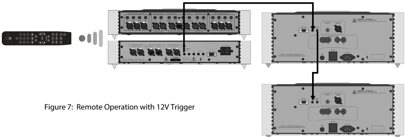
Figure 7: Remote Operation with 12V Trigger
