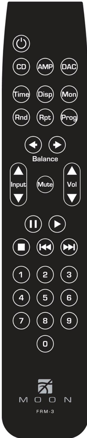
The **MOON 850P** Dual-Mono preamplifier uses the '**FRM-3**' full function, all aluminum backlit remote control (figure 5). It operates on the Philips RC-5 communication protocol and is can be used with other MOON components such as CD Players, DAC's, Integrated Amplifiers, as well as other Preamplifiers.
