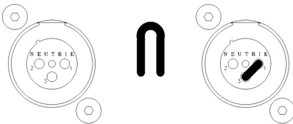
Figure 2: XLR connector without and with jumper accessory
