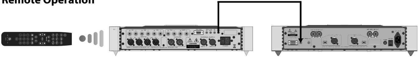
Figure 4: Remote Operation with 12V Trigger
