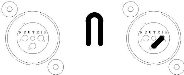
Figure 2: XLR connector without and with jumper accessory
