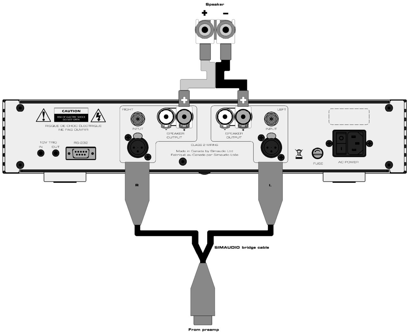
Figure 3: Bridged-Mono operation of the Nêo 330A Power Amplifier
