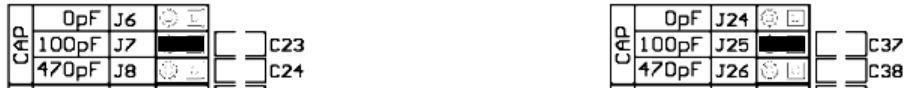
Figure 4: Left and right channel jumper banks for capacitance load adjustments at default settings
