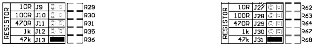
Figure 2: Left and right channel jumper banks for resistance load adjustments at default setting
