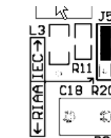
Figure 7: IEC Equalization curve jumper setting
