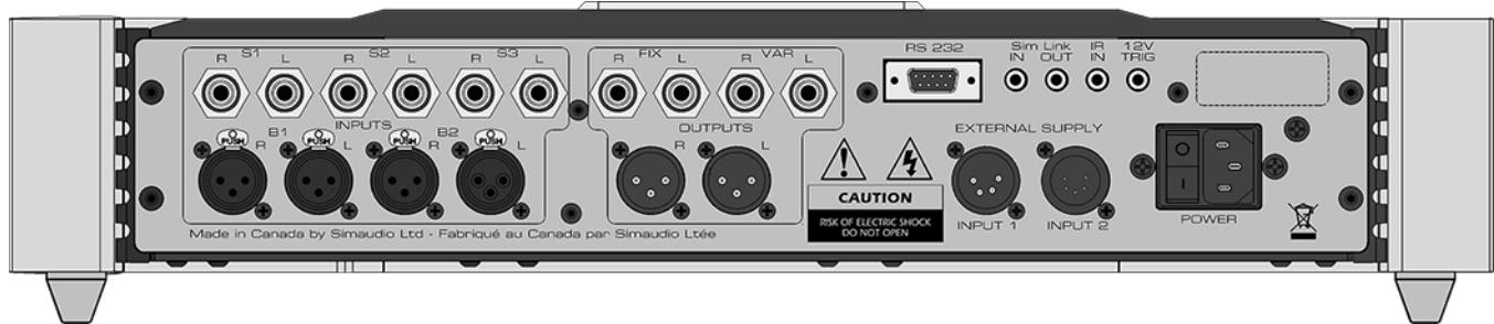
Figure 2: Rear panel of MOON 740P Preamplifier
