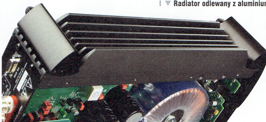
▼ Radiator odlany z aluminium.
